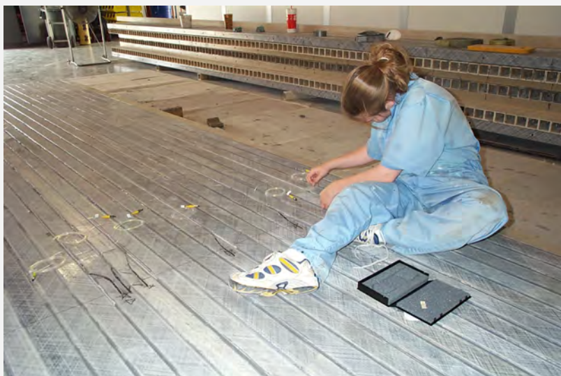
Fig. 5 Fiber optic sensors are embedded in the bottom layer of the Smart Composite Bridge during assembly. The full-scale I-beam test article is shown in the background.
