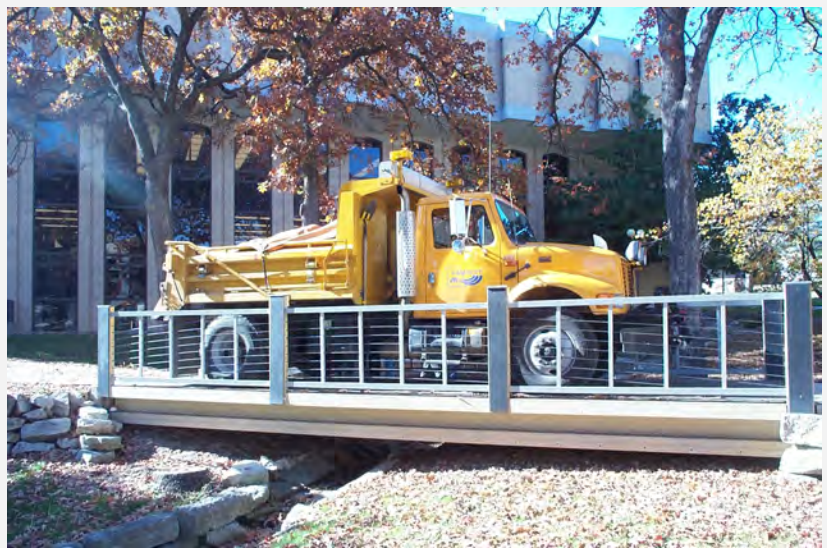
Fig. 4 Missouri S&T Smart Composite Bridge during a near-rating load test with a weighted truck.
